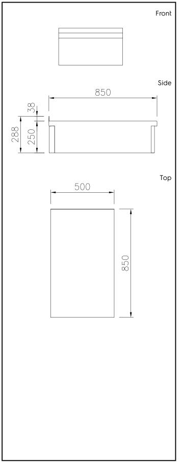
Modular Cooking Range Line thermaline 85 - 500 mm Closed Work top, 1 Side with Backsplash
